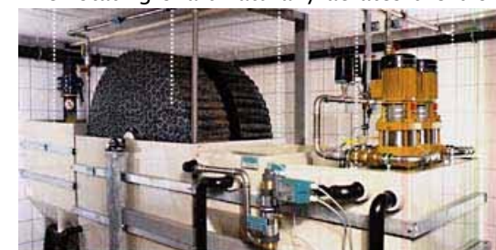
Figure 12b. Example of a rotating biological contactor
