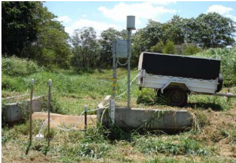
Figure 8. An example of a trailer-mounted autosampler, which is similar to the one positioned at Stuart Creek (D/S) (Photo: Faithful et al. 2007)
